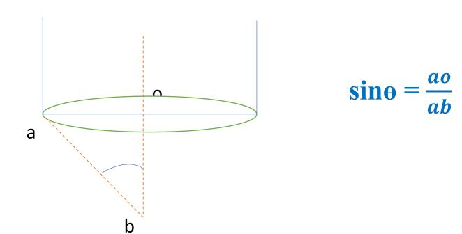
• With dry objective the value of  $\eta$  is 1, since the refractive index of air is 1, with the use of immersion oil  $\eta$  is 1.56
