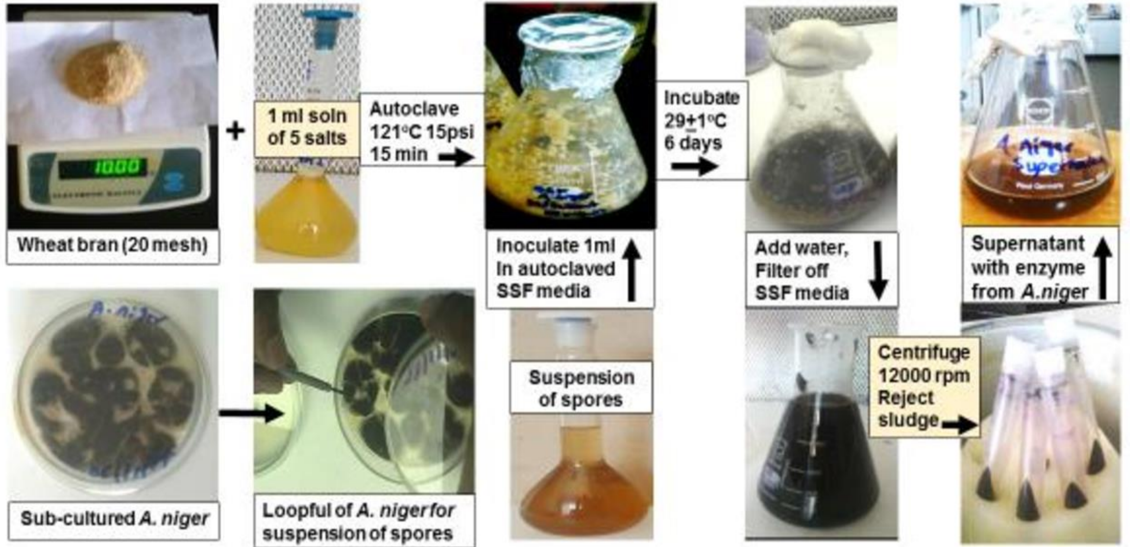
Fig. 1 Steps of Solid State Fermentation process to obtain enzyme from the fungus Aspergillus niger
